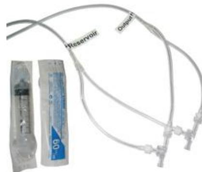
For use with our continuous infusion system or dual infusion system. Provides a dual check valve for two syringes, withdraw will pull fluid from a reservoir and infusion will output into a separate line. The kit is pre-assembled, all you need to do is plug in the syringes. Each dual check valve uses 6" of 1/8" tubing to connect to a Y connector, one for reservoir and one for output; each Y-connector has 5' of tubing to make connections to your application. Two 60cc Terumo syringes are included.
